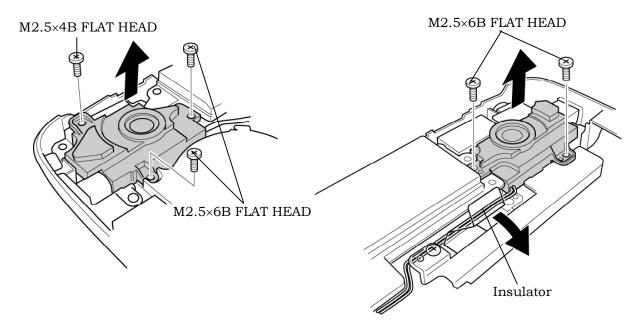
Figure 4-31 Removing the speakers
